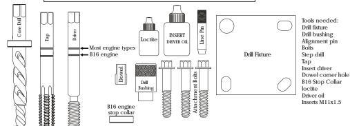
NOTE: For B16 and similar engine blocks, use the B16 spacer on core drill, and go to the first line on tap and insert driver tool. Use with blocks which have a thread depth of approx. 47mm from the top of the deck to the first thread.
